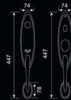
Model: 800双拉手锁 颜色: 铜本色/镀金PVD/青古铜/红古铜 Color: Original Stainless Steel/PVD/AB/AC 材质: SUS304不锈钢 Material: SUS304 Stainless Steel 表面处理: 镜光、拉丝 Finish: Polished/Satin
